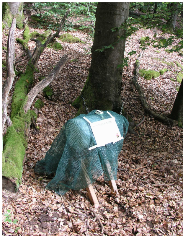
Figure 10 : A GPS collar fixed on a jerrycan of water on the support in wood with a camouflage net on it
