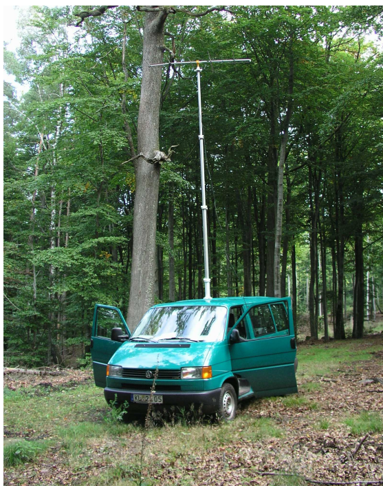
Figure 7 : The bus used for the VHF telemetry with the telescopic pole deployed
